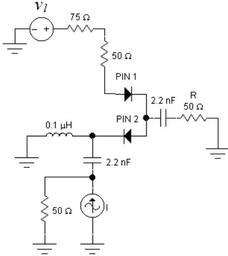
Fig. 4. Schematic circuit of the single pole single through switch using the 1SV172 diode pair.
