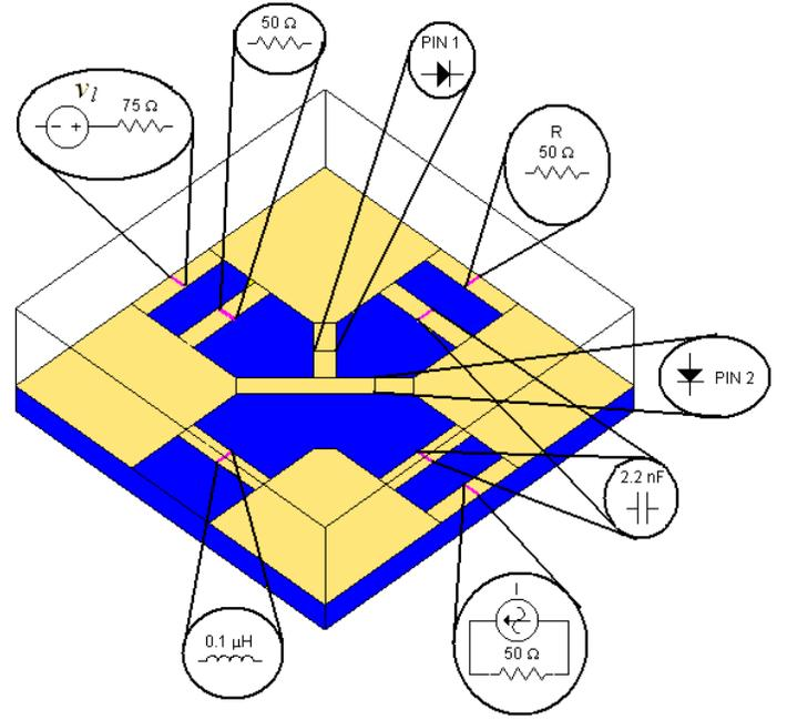
Fig. 5. Structure of the single pole single through switch using the 1SV172 diode pair.
