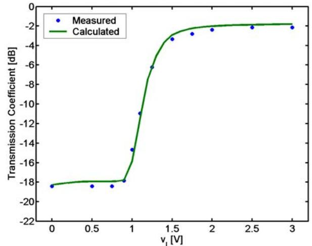
Fig. 6. Single pole single through switch transmission coefficient against DC control voltage: • measured, — calculated.
