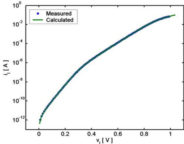
Fig. 2. IxV curve of the 1SV172 PIN diode: • measured, — fitted.
