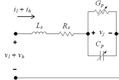
Fig. 1. Equivalent circuit model of a PIN diode.
