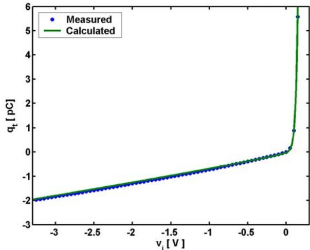
Fig. 3. QxV curve of the 1SV172 PIN diode: • measured, — fitted.
