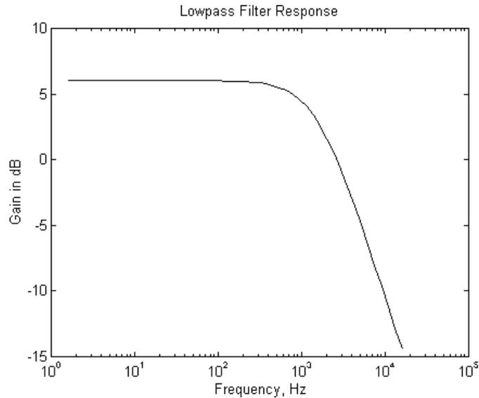
**Figure 7.19** Magnitude Response of an Active Lowpass Filter
