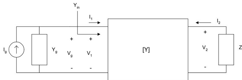
**Figure 7.16** A Terminated Two-Port Network with y-parameters Representation
