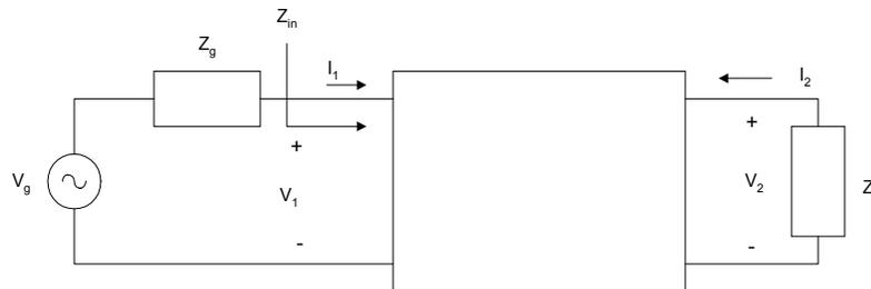
**Figure 7.15** Terminated Two-Port Network
