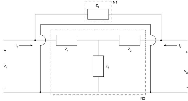
**Figure 7.11** An Alternative Representation of Bridge-T Network
