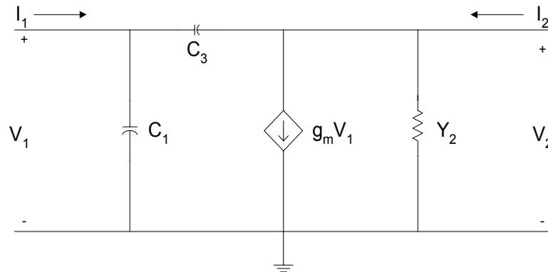
Figure 7.4 Simplified Model of a Field Effect Transistor
