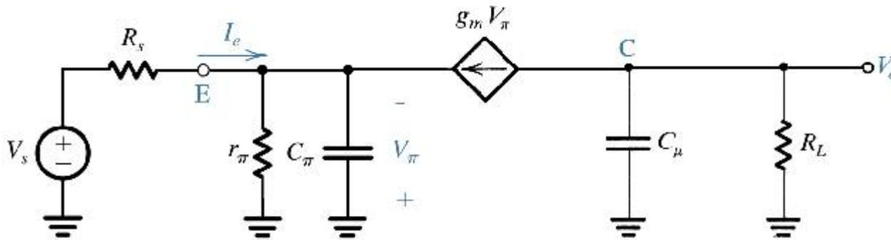
$$\omega_{P1} = \frac{1}{C_{\pi}(r_{\pi} \parallel R_s)}$$
