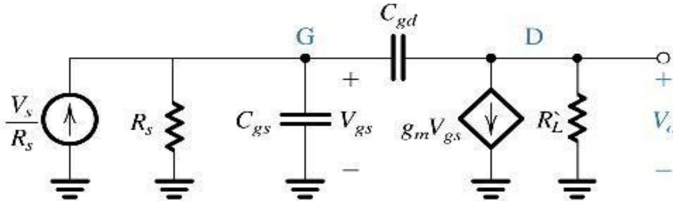
$$\frac{V_o(s)}{V_s(s)} = A_M \frac{1 - \frac{s}{g_m / C_{gd}}}{1 + s R_s [C_{gs} + C_{gd} (1 + g_m R'_L) + C_{gd} (R'_L / R_s)] + s^2 C_{gs} C_{gd} R_s R'_L}$$
