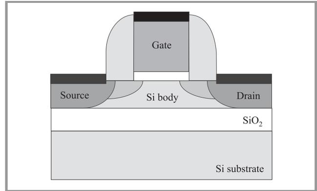
Fig. 5. A cross section of a SOI MOSFET.
