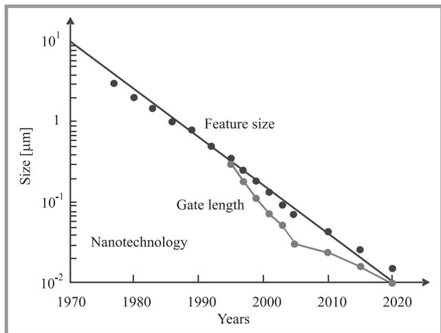
Fig. 8. Feature size as a function of time (data after [45]).
