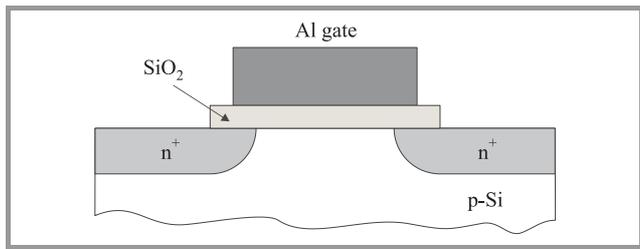
Fig. 4. A cross section of a metal-oxide-semiconductor transistor.
