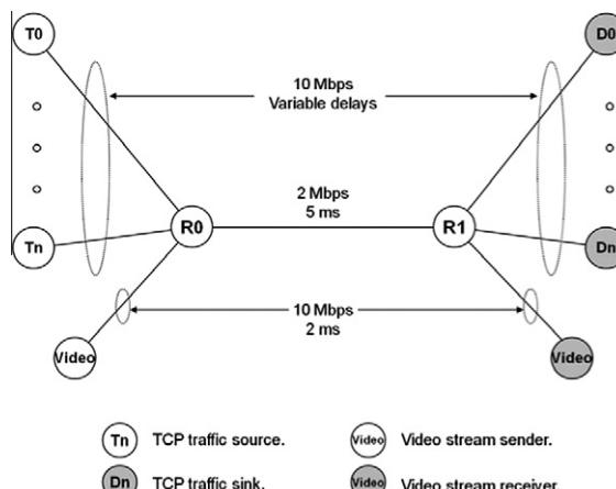
**Fig. 1.** Simulated network topology.
