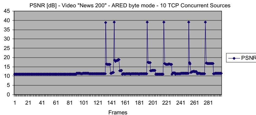
**Fig. 20.** Video sample news 200 – PSNR under ARED byte-mode technique, 10 concurrent TCP sources.
