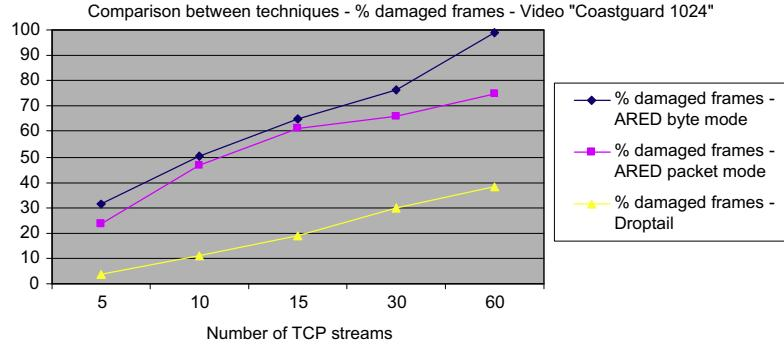
**Fig. 14.** Video sample coastguard 1024 – percentage of damaged video frames.
