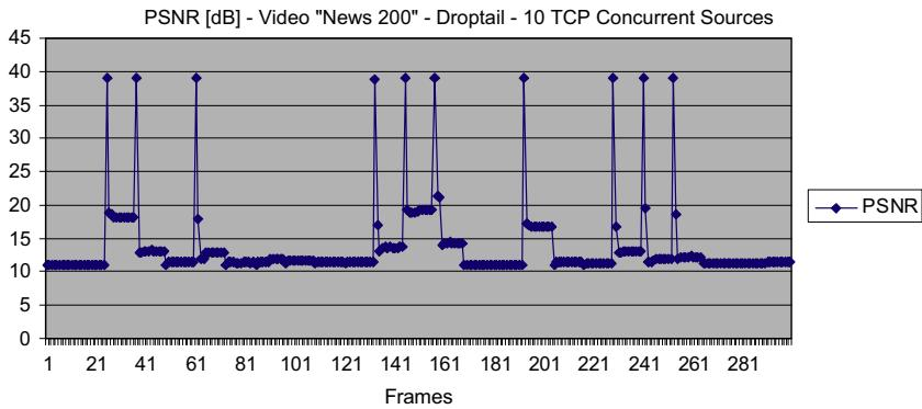
Fig. 19. Video sample news 200 – PSNR under drop-tail technique, 10 concurrent TCP sources.
