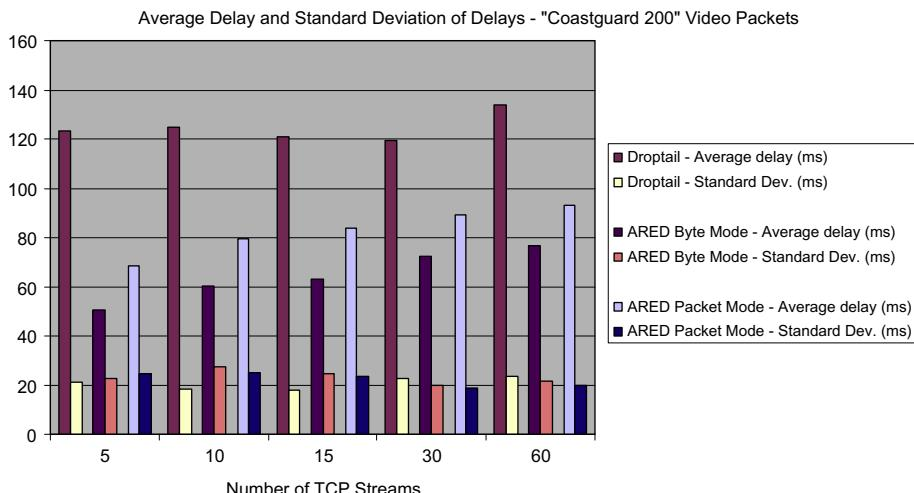
**Fig. 4.** Video sample coastguard 200 – average delay and standard deviation.
