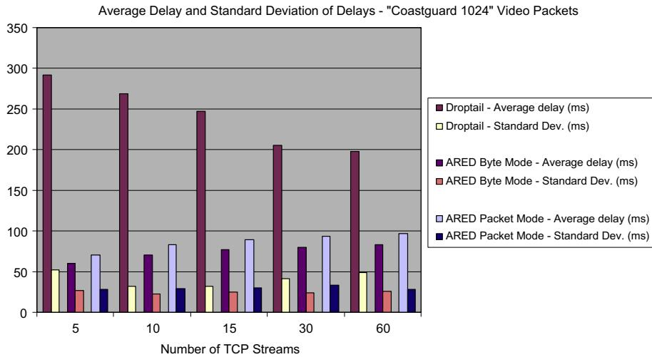
**Fig. 6.** Video sample coastguard 1024 – average delay and standard deviation.
