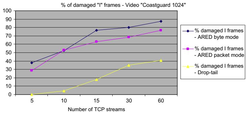
Fig. 18. Video sample coastguard 1024 – percentage of damaged 'I' frames.
