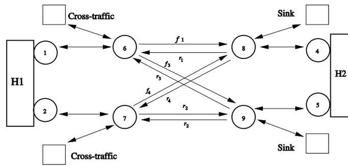
Figure 14 Network topology in simulations - SCTP and cross-traffic
