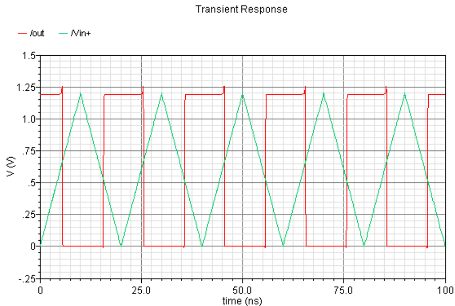
Figure 28 - Simple NMOS comparator operation
