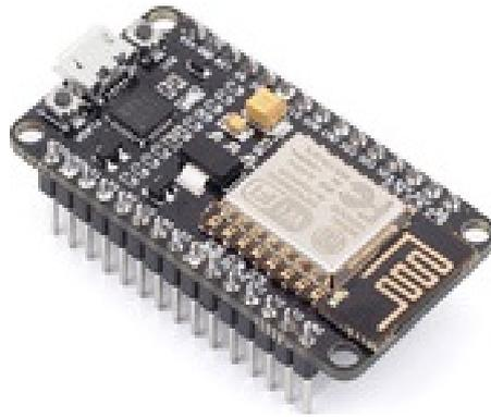
Figura 2.9: NodeMCU
