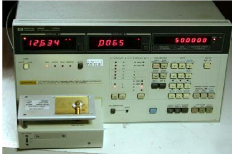
Figura 18: RF Impedance Analyzer Agilent HP4191A (O autor, 2018).
