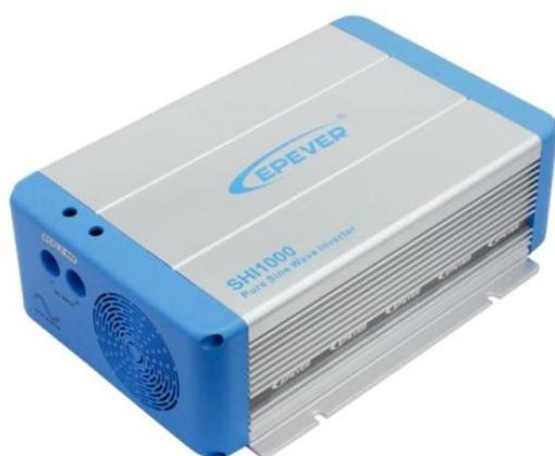
SHI series is a pure sine wave inverter which can convert 12/24/48Vdc to 220/230Vac 50/60Hz based on full digital and intelligent design. It features high reliability, high efficiency, concise outline, small volume, easy installation and operation. The inverter can be applied in many fields, such as household appliances, electric tools and industrial devices etc, especially for solar photovoltaic power system.
