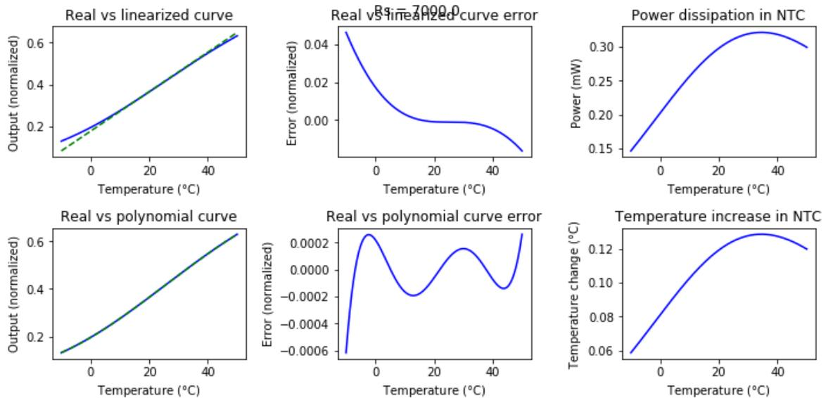
(a) Simulação com  $R = 7k\Omega$
